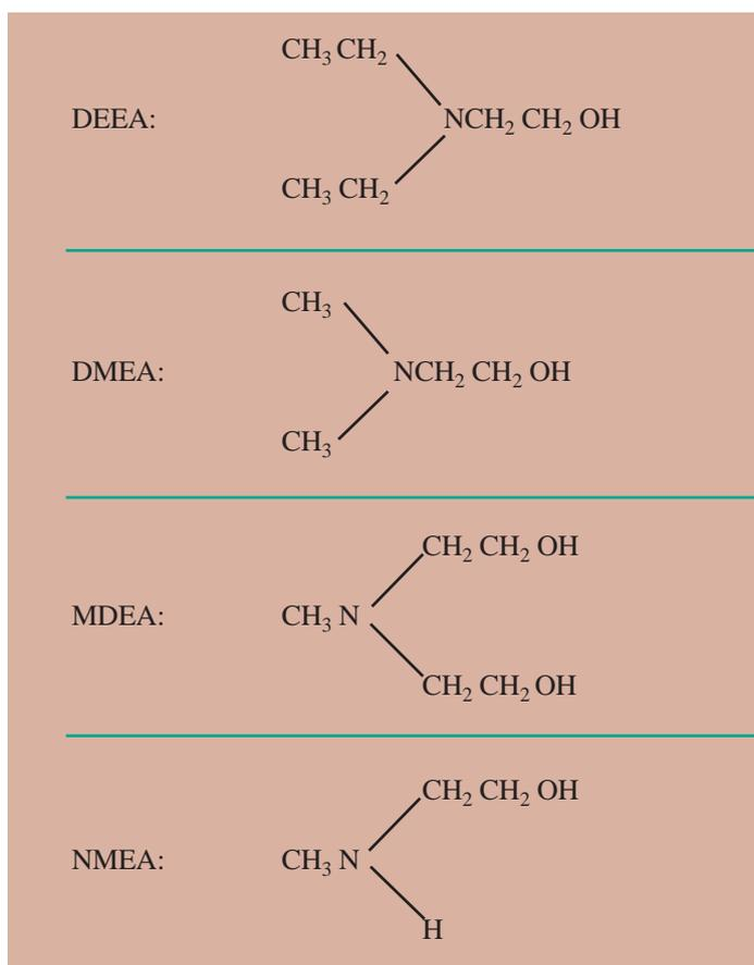
Alkyl alkanolamines are liquids at room temperature. N-methylethanolamine has the highest freezing point of this family at  $-5^{\circ}\text{C}$ , while N,N-diethylethanolamine has the lowest freezing point at  $-78^{\circ}\text{C}$ . They are hygroscopic, mildly alkaline, and completely water soluble. For these reasons, they are often used for pH control in such markets as water treating and coating applications.
