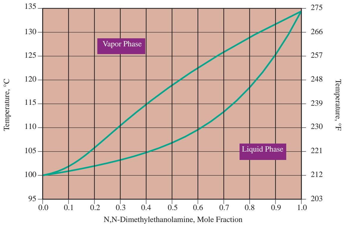
**Figure 5** Vapor – Liquid Equilibria of Aqueous N-Methylethanolamine Solutions at 760 mm Hg
