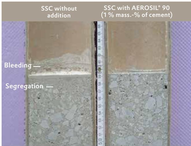
However, one should take into account, that use of AEROSIL® fumed silica grades with high specific area (AEROSIL® 200, AEROSIL® 300) increases the viscosity of wet concrete. If viscosity increase has to be limited, AEROSIL® grades with surface area about 100 m<sup>2</sup>/g, for example, AEROSIL® 90 should be used.
