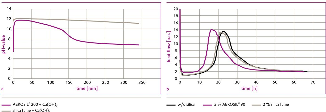
Reactivity and morphology of AEROSIL® fumed silica and SIPERNAT® specialty silica are beneficial for consistency of ultra-high performance concrete (UHPC). As demonstrated in [3], a consistent compressive strength of 150 MPa could be achieved after 28 days. UHPC is a high-density concrete, which has outstanding mechanical properties.
